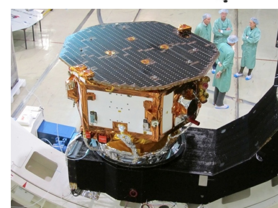
Fig. 7: Picture of LISA Pathfinder satellite during OSTT campaign (On-Station Thermal Tests) in which conditions close to space environment are obtained. Credit: Airbus Defence and Space GmbH, Friedrichshafen.
