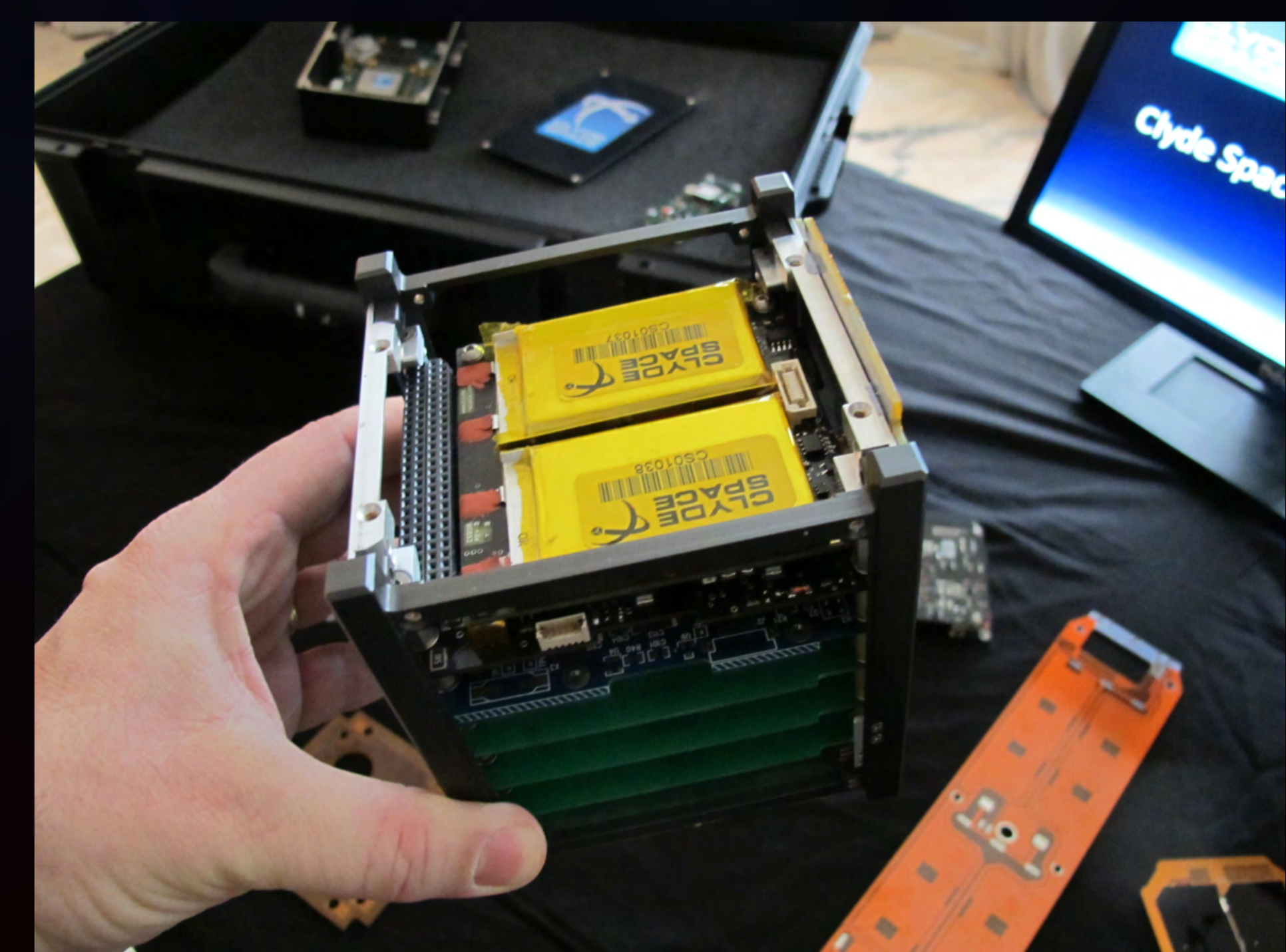
1U CubeSat structure from the company Clyde Space
