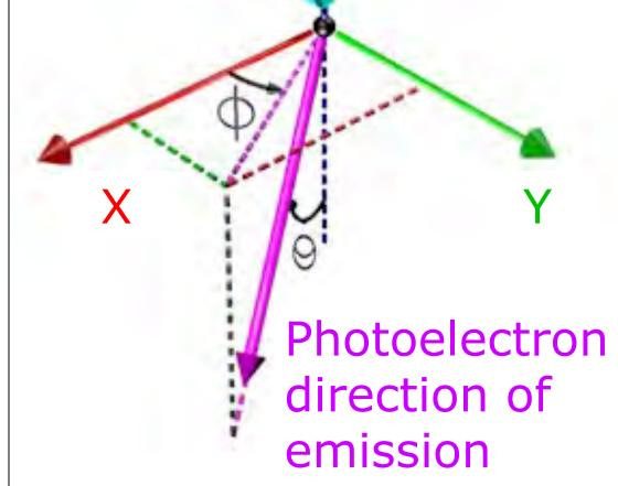
Emission probability modulated by  $cos(\Phi)^2$ : The photo-electron has a greater probability of being ejected at the angle  $\Phi=0$
